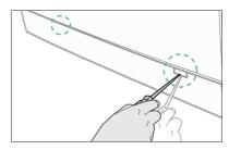
**3.** Unscrew the emergency drain cap by turning left. Grip the cap on the end of the emergency drain tube and slowly pull it out about 15 cm.
